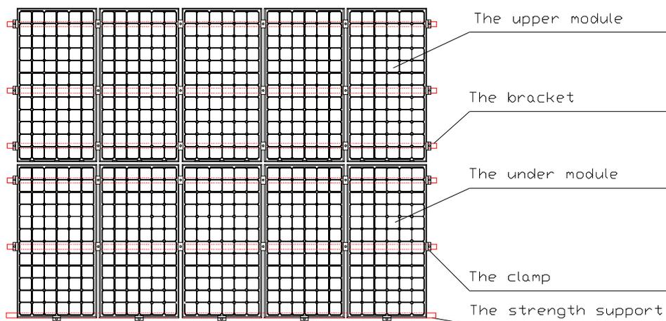
FIG 3 Schematic diagram of reinforcement mounting of module
