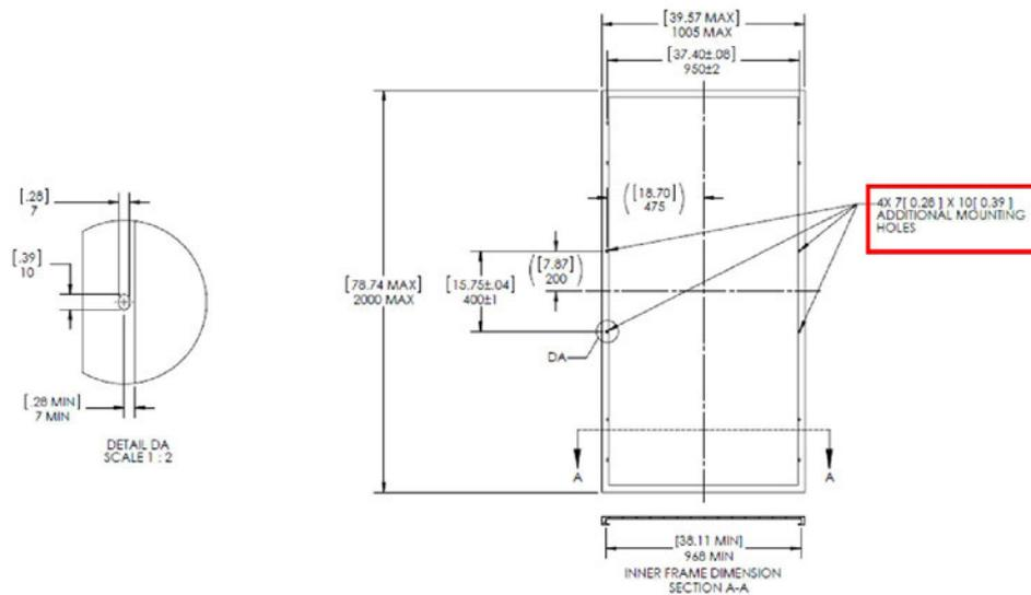
FIG 7. NEXTracker mounting holes at 400mm short rails
