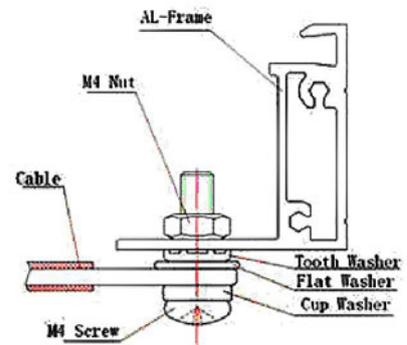
FIG 8-b Grounding method
